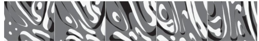
Odd and even half-frames superimposed semitransparently (1/25 second in length). Superimposing white fields over black fields produces gray. White superimposed over white and black over black remains white or black. This provides an example of what happens to the half-frames in progressive-scan mode. They are assembled or merged and lengthened to 1/25 second.
